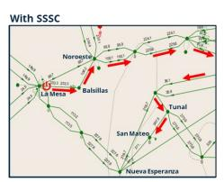
Hence, the placing FACTS equipment in the upper ring of the San Mateo-Nueva Esperanza line successfully redirected power flow and deferred the need for conventional transmission line duplication.
