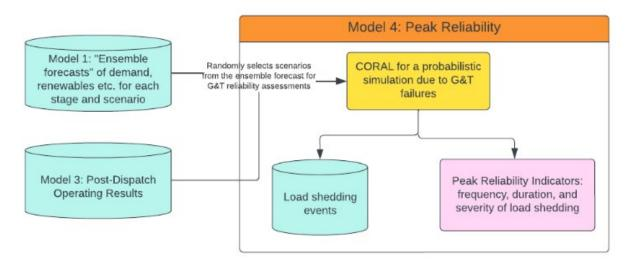
The methodology for estimating peak reliability indicators builds upon the outcomes of the composite generation-transmission reliability model (CORAL). CORAL employs Monte Carlo simulations, randomly sampling failure and repair processes across all generation and transmission components to determine the availability of generation and transmission resources for each hour within a selected peak demand block.
