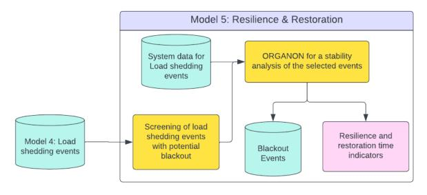
Finally, model 5 will consider the peak reliability simulation results and identify scenarios where load interruptions occurred and select those with a high probability of causing blackouts and model the fault
