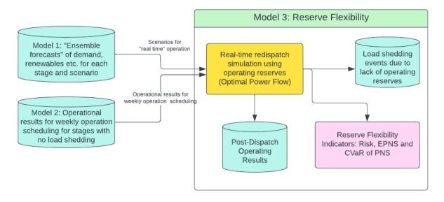
The reserve flexibility indicators aim to emulate real-time system operation, specifically assessing whether the reserves scheduled during weekly operational planning are sufficient to accommodate deviations between forecasted and actual system conditions, known as the "true up" process.
