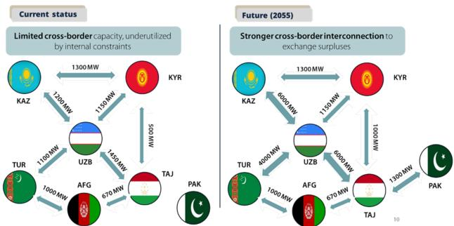
The analysis also shows that current interconnection limits are a key constraint. Transmission upgrades — especially east-west corridors and north-south links to Pakistan and Afghanistan — are required to enable efficient seasonal balancing and export flows. Hydrological diversity can be monetized only if physical exchange infrastructure is in place.
